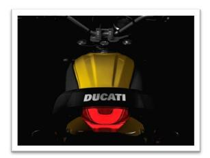
At the rear, instead, lies a full-LED unit. This gives off a suffused light and features a technology unprecedented on motorcycles; this 'soft' effect is, in fact, achieved by combining an opaque light-diffusing lens with a 12-LED electrical card (18 LEDs when the brake is applied).
